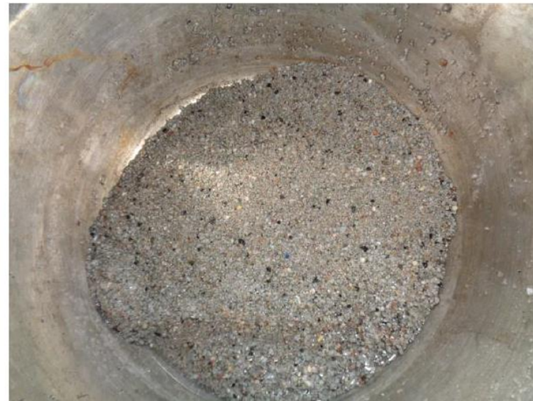
Fraction 0.25 - 2 mm (wet) after shock wave treatment (150 discharges)
