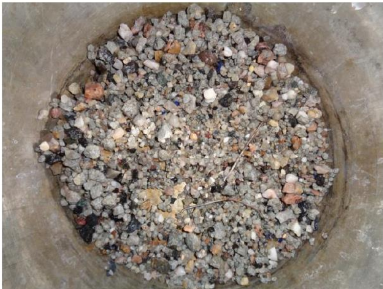
Fraction 2 - 8 mm (moist) after shock wave treatment (150 discharges)
